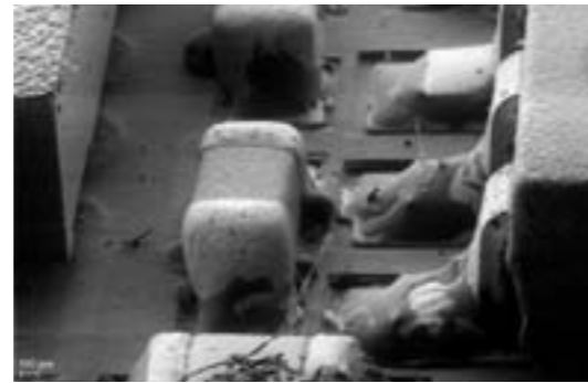
Low magnification SE image of a PCB with SMD in VP mode (16 kV and 36 Pa chamber pressure). True SE imaging without destroying the PCB.
