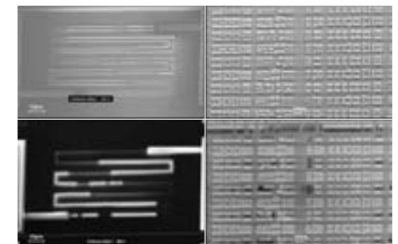
Two examples of potential contrast imaging with the SUPRA® 55. Images on the left are of the same area showing signal flow, with the top image through 2 µm passivation layer. Image top left topographic of the IC surface. Image bottom right shows active components in voltage contrast.
