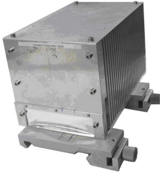
Figure 3.2: Medipix 2 detector: the area behind the aluminum strip can contain up to 5 sensors.
