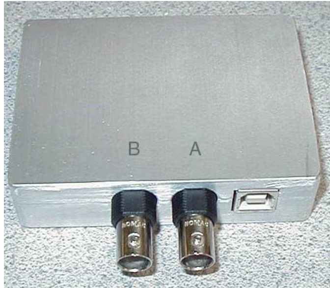
Figure 3.3: Hardware Correlator Flex01-08D, with two input connections and an USB output.
