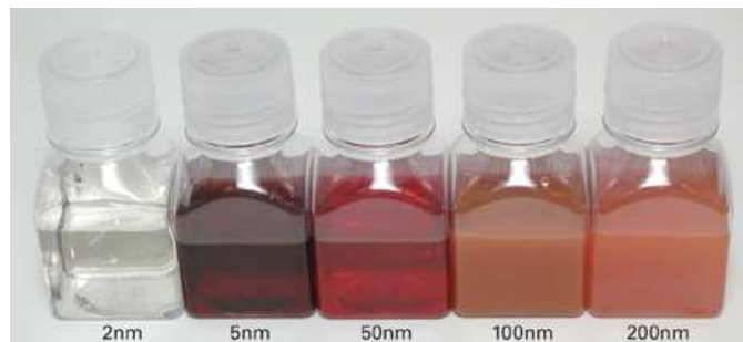
Figure 1.1: Gold nanoparticles suspended in water; the radius of the particles determines the colour of the suspension. From [2].
